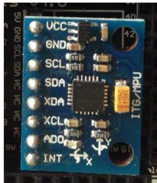
Figura 3. 7: Giroscopio MPU 6050
