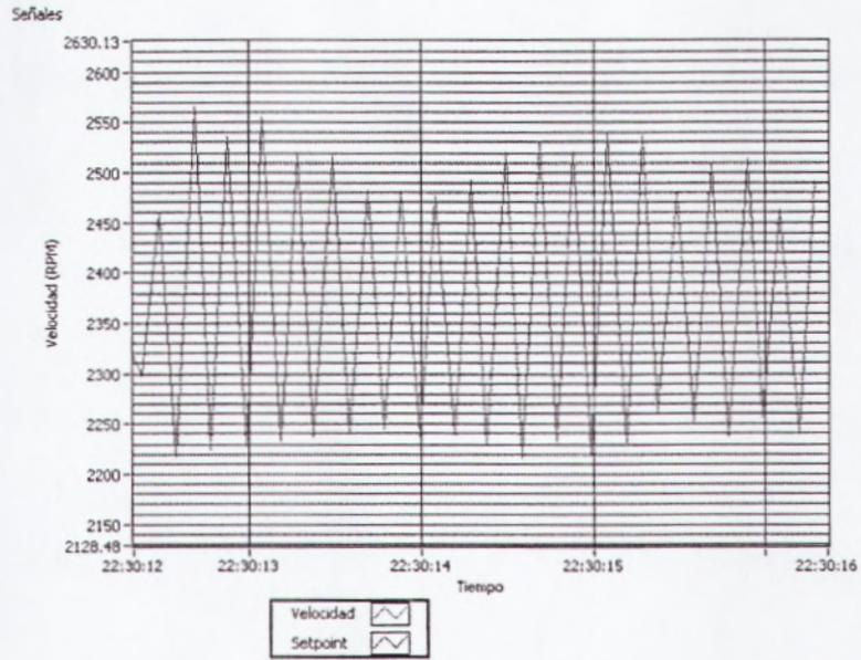
Figura 4.42:  $F_{cr} = 4.9 \text{ Hz}$   $P_{cr} = 1/4.9 = 0.2 \text{ segundos}$
