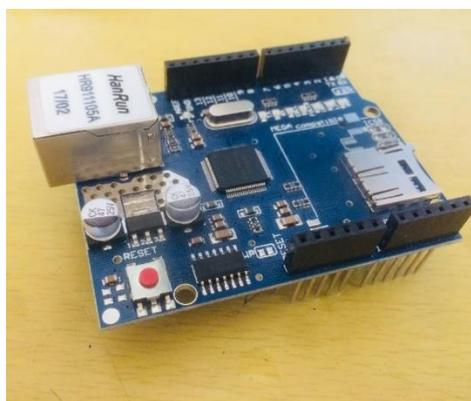
Figura 3. 6: Shield Ethernet.
