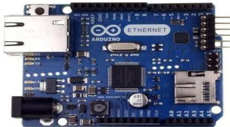
Figura 3. 12 Arduino Ethernet
