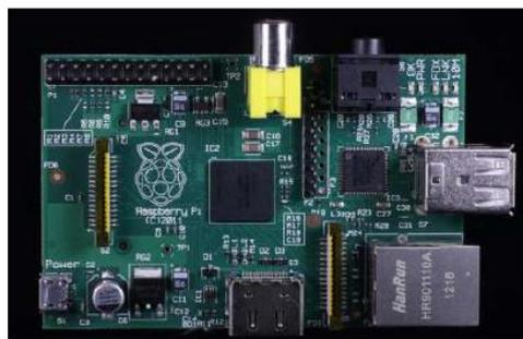
Figura 2. 11: Raspberry Pi Modelo B
