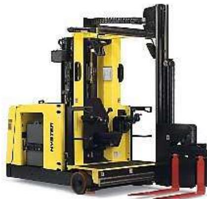
*Figura 2.5: Montacargas Trilateral Hyster V30-35ZMU series
