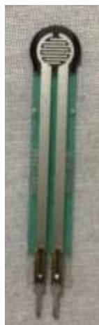
Figura 2.7 Sensor FSR 400
