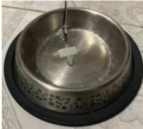
Figura 3.34 Sensor FSR 400 instalado
