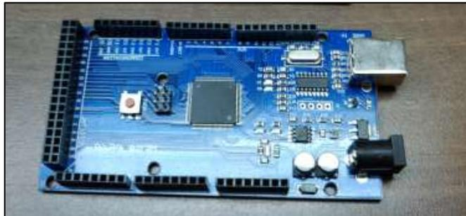
Figura 3. 8: Tarjeta Arduino Mega 2560
