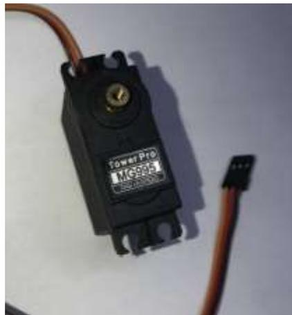
Figura 3. 8: Servomotor MG995.
