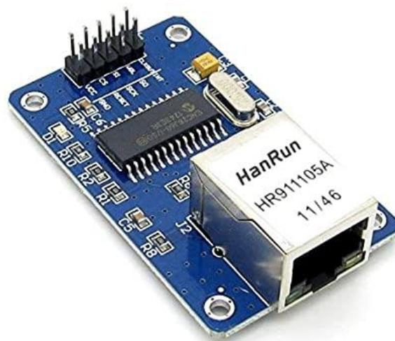
**Figura 3. 4** *Módulo Ethernet Arduino Enc28j60*
