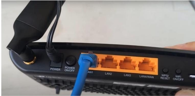
**Figura 3.6:** Puertos LAN y Cable Ethernet Cat6 LAN UTP
