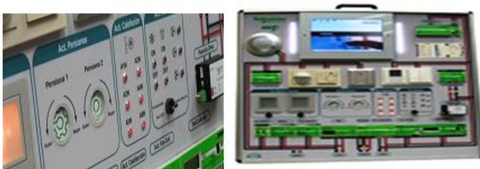
**FIGURA 3.7 PANEL DOMÓTICO KNX AVANZADO.**
