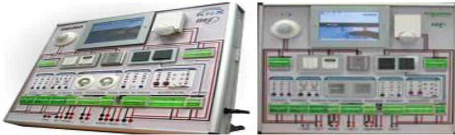
**FIGURA 3.6 PANEL DOMÓTICO KNX INTERMEDIO.**
