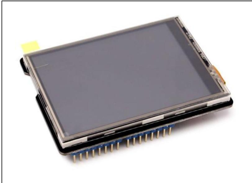
Figura 2.15 Shield de pantalla TFT 2.8 “
