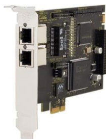
Figura 5.47 – Tarjeta PCI Express, Digium TE220 2 puertos (T1/E1)
