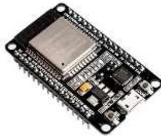
**Figura 29.** Arduino ESP32 (Hoddie & Preder, 2020)
