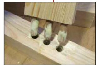
ANCLAJE DE TAPA FRONTAL CON TARUGOS O CON MINIFIX
