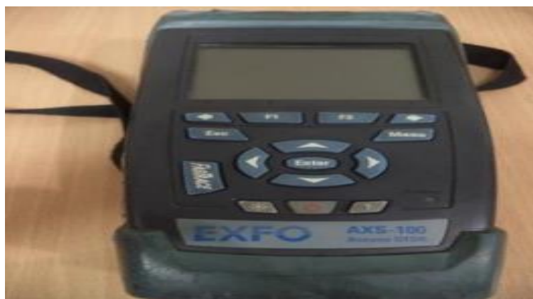
Figura 2.25: OTDR EXFO – 100 Access OTDR Fuente: (Lorenti, 2014)
