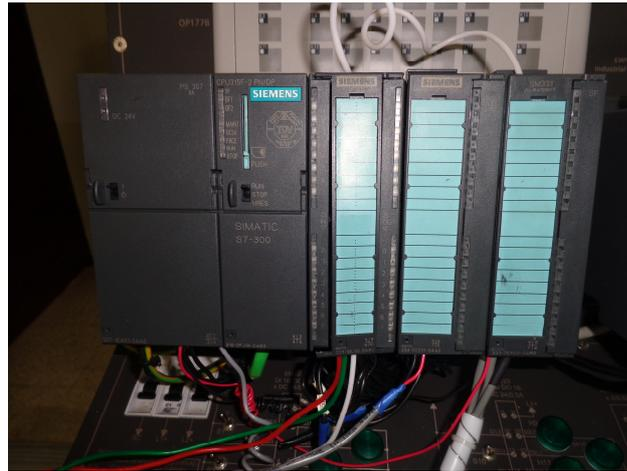
**Figura # 62 PLC step 7 300, CPU 315F-2PN/DP.
