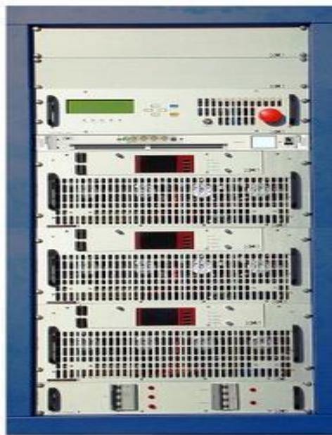
Figura 4.5 *Transmisor de TV digital MOT 2000/2400(OMB)*
