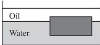
31. A layer of oil with density  $800 \text{ kg/m}^3$  floats on top of a volume of water with density  $1,000 \text{ kg/m}^3$ . A block floats at the oil-water interface with  $1/4$  of its volume in oil and  $3/4$  of its volume in water, as shown in the figure above. What is the density of the block?
