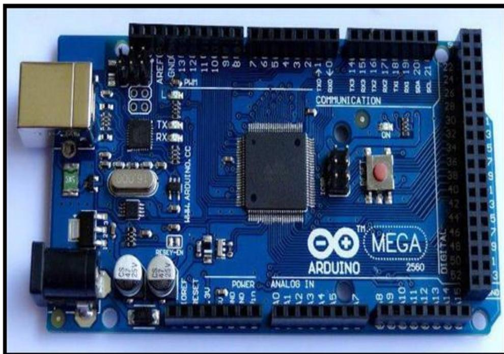
Figura 3. 2: Arduino mega 2560
