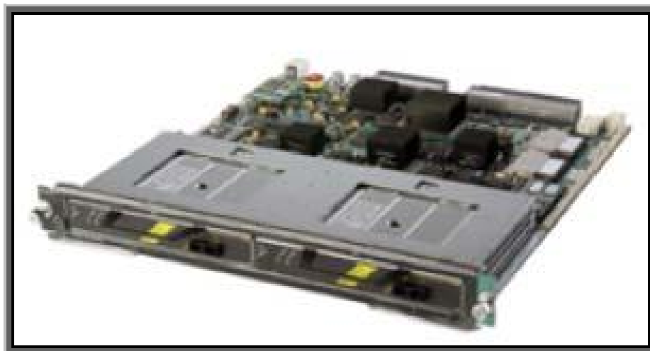
Figura 61: Tarjeta Enhanced FlexWAN Module (WS-X6582-2SPA) (8)
