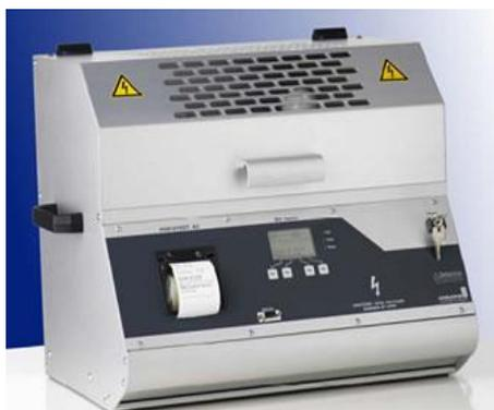
**FIG. 5.3 CHISPÓMETRO**
