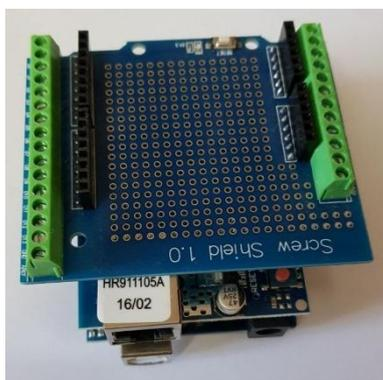
**Figura 3. 36: Tarjeta Screw Shield 1.0**
